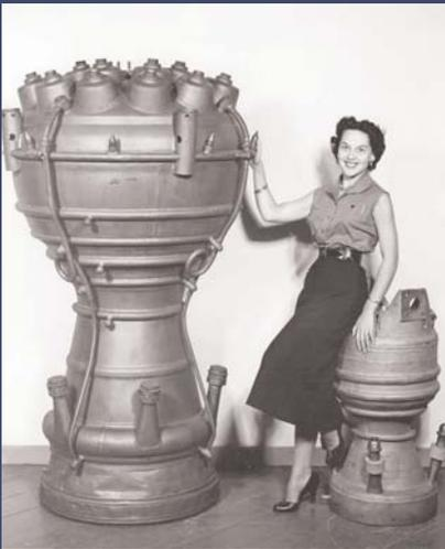
Photograph of Reaction Motors, Inc., rocket engine for the Viking missile (left) as compared to an engine from the German V-2 rocket from World War II. Photo c.1951 (author's collection).
