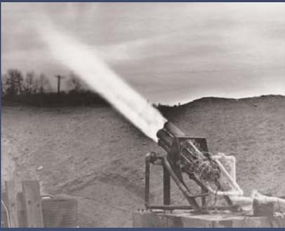
**Photograph of Reaction Motors, Inc., Model 6000-C4, four-cylinder, liquid propellant rocket engine, in operation on test stand at Pompton Plains, N.J., c.1949. This was the engine that would power the Bell X-1, breaking the sound barrier.** (author's collection)
